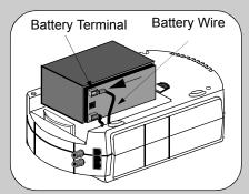
Insert the battery back into the compartment. Slide the plastic battery cover in place until the two tabs lock into place.
